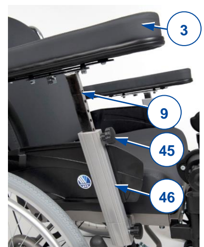
Figure 7 Adjusting armrest height
